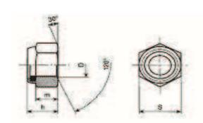
MATERIALE CORPO DADO: ACCIAIO AD MEDIA RESISTENZA CLASSE: 6S MATERIALE: (INSERTO): POLIMIDE CARICO DI DUREZZA MIN: 89 HRB FILETTATURA METRICA ISO GRADO MEDIO: 6h DIN 13/12<15 FINITURA SUPERFICIALE: ZINCATI BIANCHI
