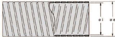
Flexible double hose made of galvanized steel or AISI 304 stainless steel.
